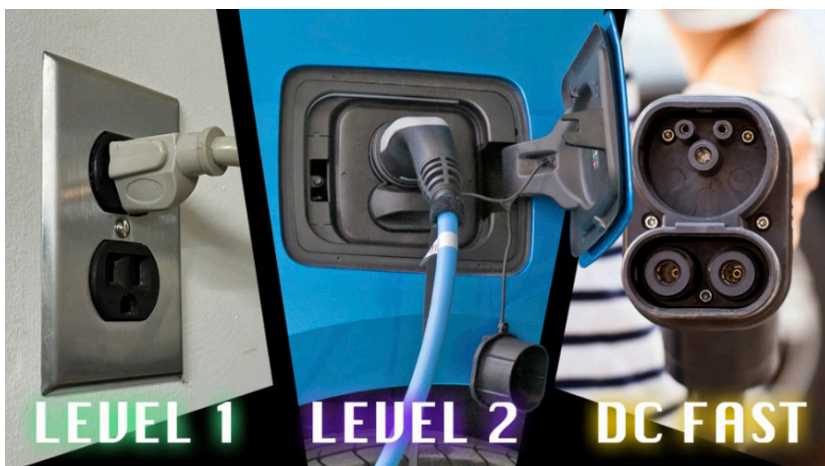
Figure 7-5: Electric Vehicle Charging Levels
