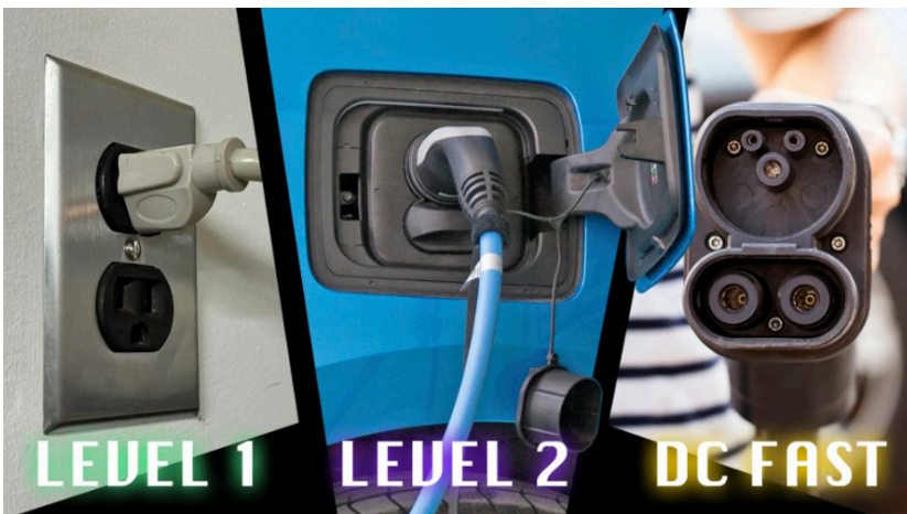
Figure 7-5: Electric Vehicle Charging Levels
